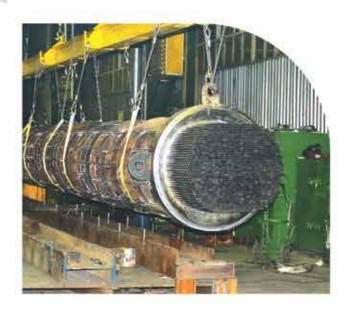
In refi-neries, Re-boilers are used as a type of shell and tube heat exchangers to reheat the condensate products at the bottom of Distillation Tower and return them vaporized to the distillation tower. Re-boilers are also designed and manufactured by MAPNA Boiler.
